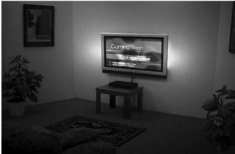
Fig. 1: View looking into the experimental test space. Surrounding illumination was presented along the left and right side of the television display
