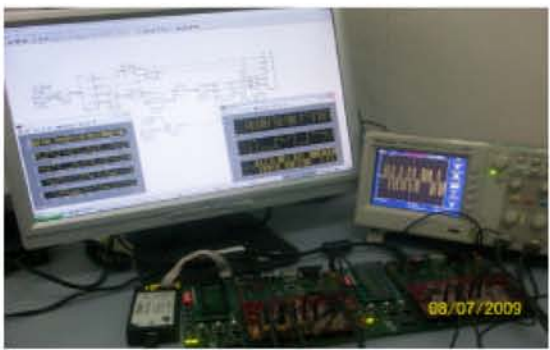
Fig. 8: Physical assembly of SDR transmitter and receiver
